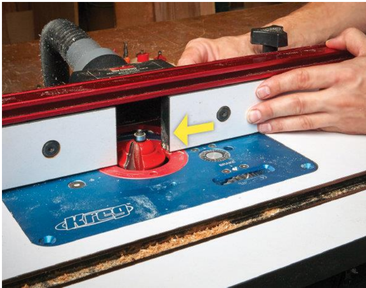
Setting the gap in the fence to match the router bit
